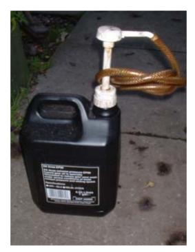
Once the gearbox is full, the oil will start to come back out of the filler aperture; now you can replace the filler plug. Remember, you can check the oil level in the gearbox at any time by removing this plug....just allow time for the oil to settle after a run....and top it up as necessary.
